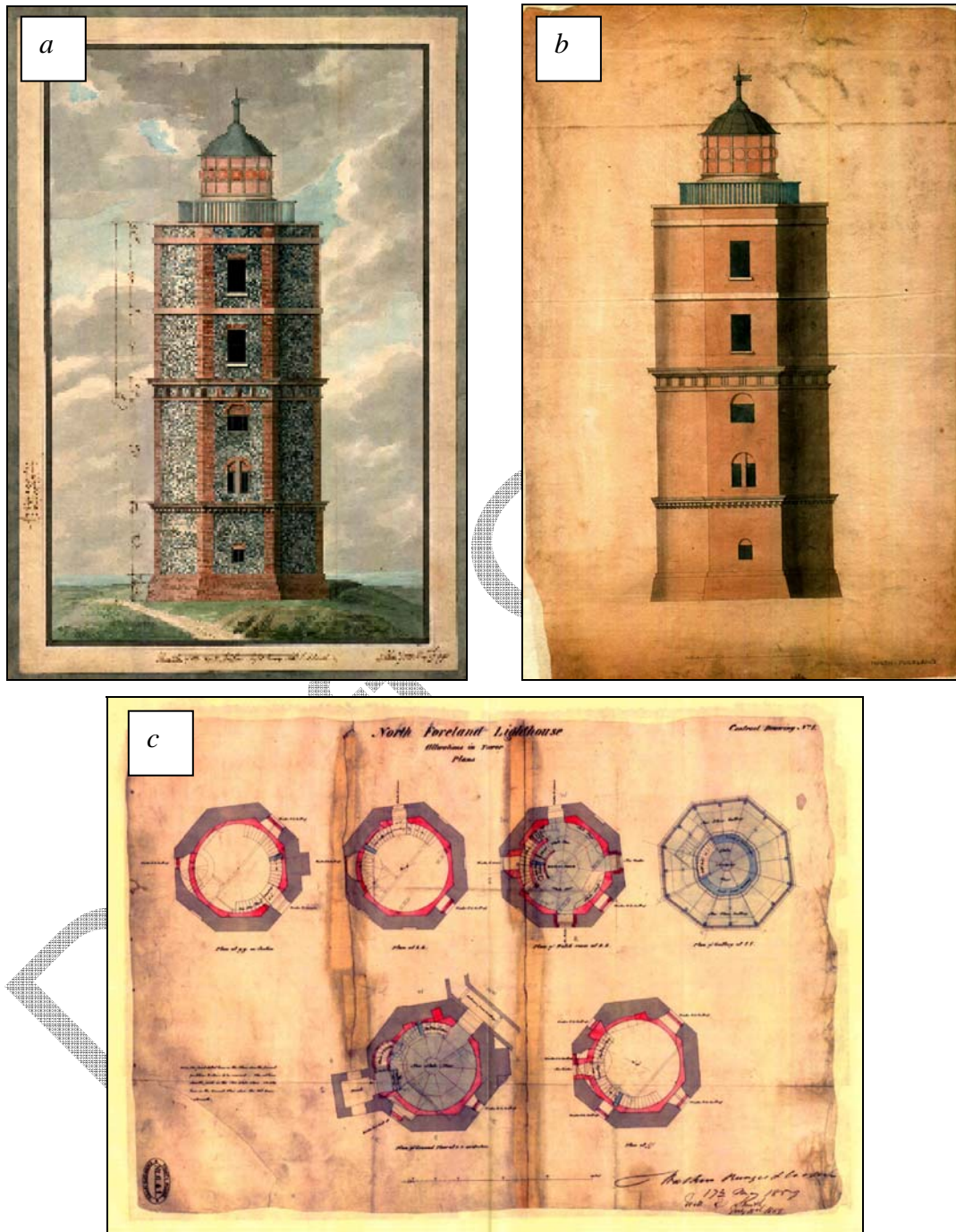
Figure 5: Historic plans and drawings of North Foreland lighthouse provide a valuable record of significant structural changes that have had a major impact on present-day building conditioning. (a) The original flint and brick finish of the tower, (b) subsequent rendering of the exterior of the tower and, (c) construction of a rounded internal structure within the original octagonal tower which has given rise to considerable stresses between different masonry materials and problems related to moisture movement and reduced breathability.
