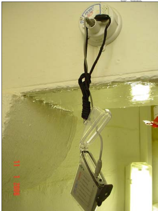
Figure 17a: HOBO data-logger in situ at North Foreland Lighthouse
